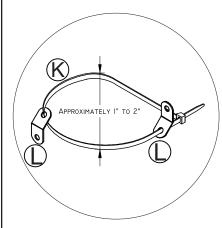
Once the clips are secure and tight, place the furniture with clips as close to the wall with clip. Then attach the cable tie (K) as shown, making sure it 'locks' and pulls together. If you wish, you can cut the top end of the tie to conceal
