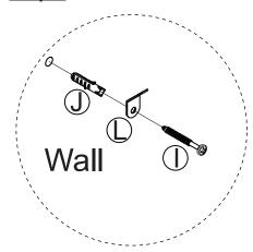
Attach the second metal clip (L) to the wall anchor (J) (If you can not use a wall stud) and screw (I) as a shown
