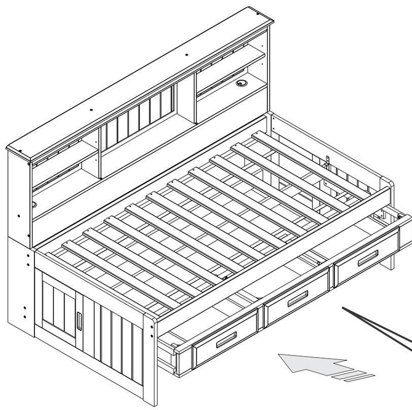
Simply slide the Drawer unit on the elevation Stick
