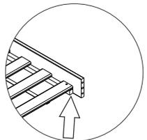
Always start assembling slat kit flush with cleat
