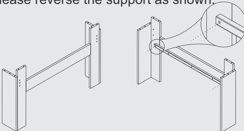
Note: If the support is not reversed as shown above, the 6 drawer unit will not fit under the bed as it will interfere with the unfinished strip.
