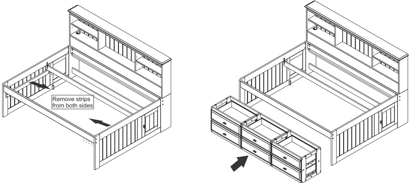
Note: If the support is not reversed as shown above, the 6 drawer unit will not fit under the bed as it will interfere with the unfinished strip.
