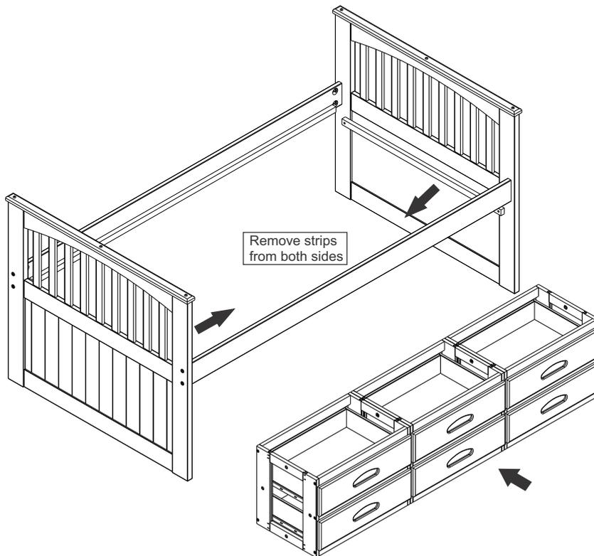
Note: If the support is not reversed as shown above, the 6 drawer unit will not fit under the bed as it will interfere with the unfinished strip.
